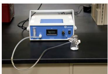
Halimeter and flask with filter paper. The filter paper was wetted with 2ml of *P. gingivalis* culture. VSCs were measured by inserting the rubber stopper into the flask and recording the maximal reading (occurred within 5 seconds). The filter was rinsed for 30 seconds with 20ml of a test rinse, the rinse was poured out and the post-rinse reading recorded.
